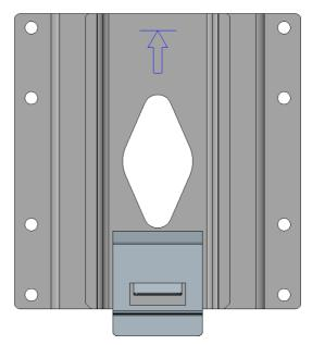
Slide the AP onto the bracket arms and secure the AP to the bracket using the screw on the side of the mounting bracket.
