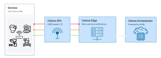
The system consists of the essential functions detailed in Figure 1: System Architecture. The Celona Orchestrator performs AP authentication, validates the AP's serial number, determines the network the AP needs to connect to and finally directs the Celona AP-12 to the serving Celona Edge.
